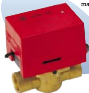
A cam enables the valve to be activated manually when there is a power cut, as well as for the filling, bleeding or emptying of the installation. If, for any reason, there is a power supply failure, the valve automatically returns to the closed position.
